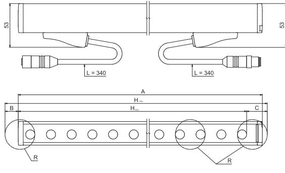
$H_{PFE}$  Effective protective field height = 1217 mm H<sub>PFN</sub> Nominal protective field height = 1200 mm
