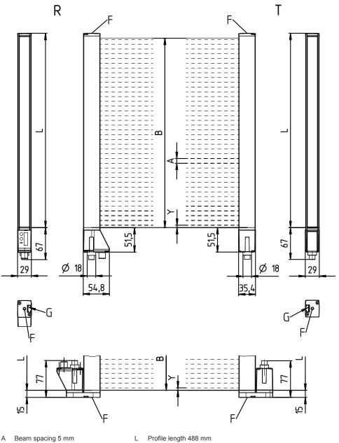
Beam spacing 5 mm А В Measurement field length 480 mm
