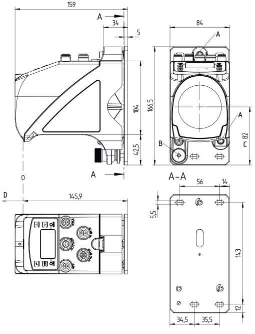
A M5 screw for alignment
