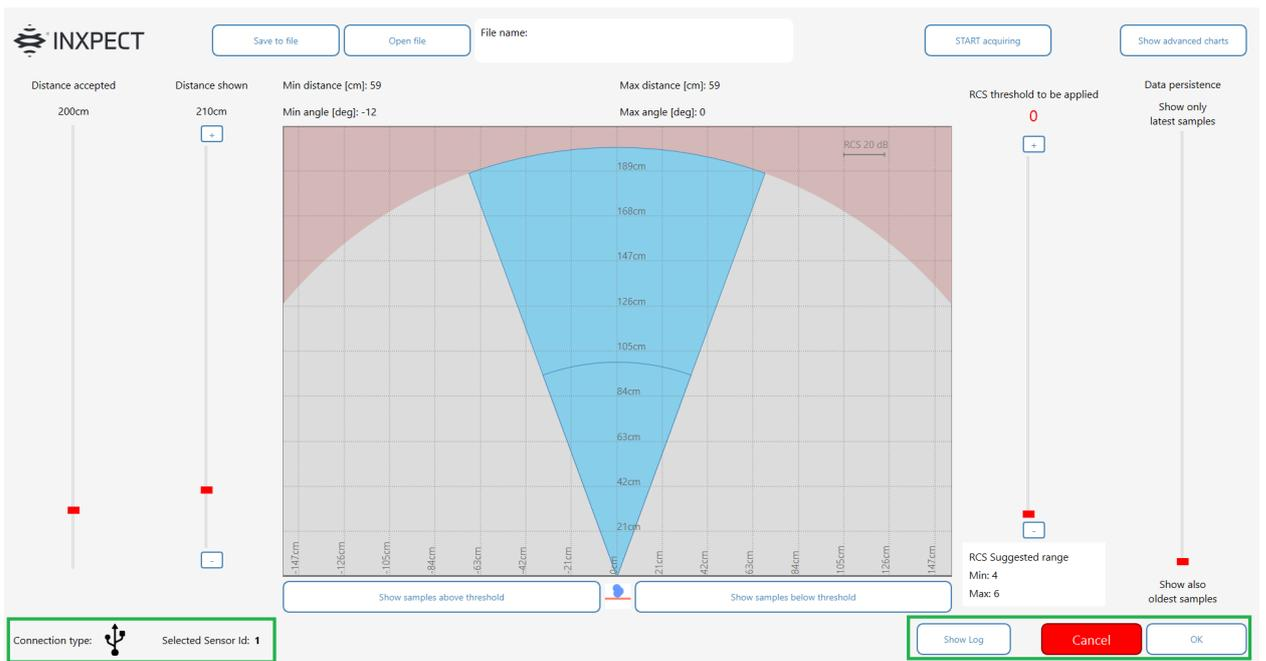
Figure 13 RCS Reader Tool: USB connection
