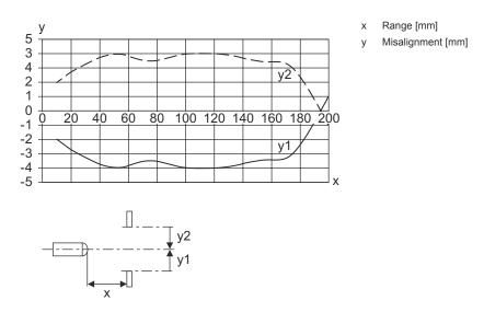
Typ. response behavior at 90% diffuse reflection (focusing distance 400 mm)
