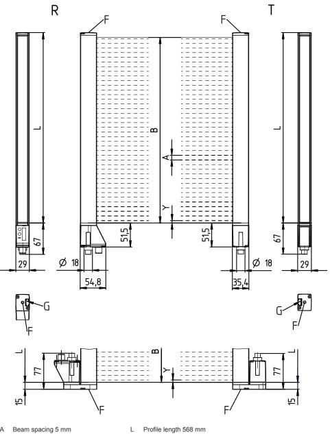
Beam spacing 5 mm А В Measurement field length 560 mm
