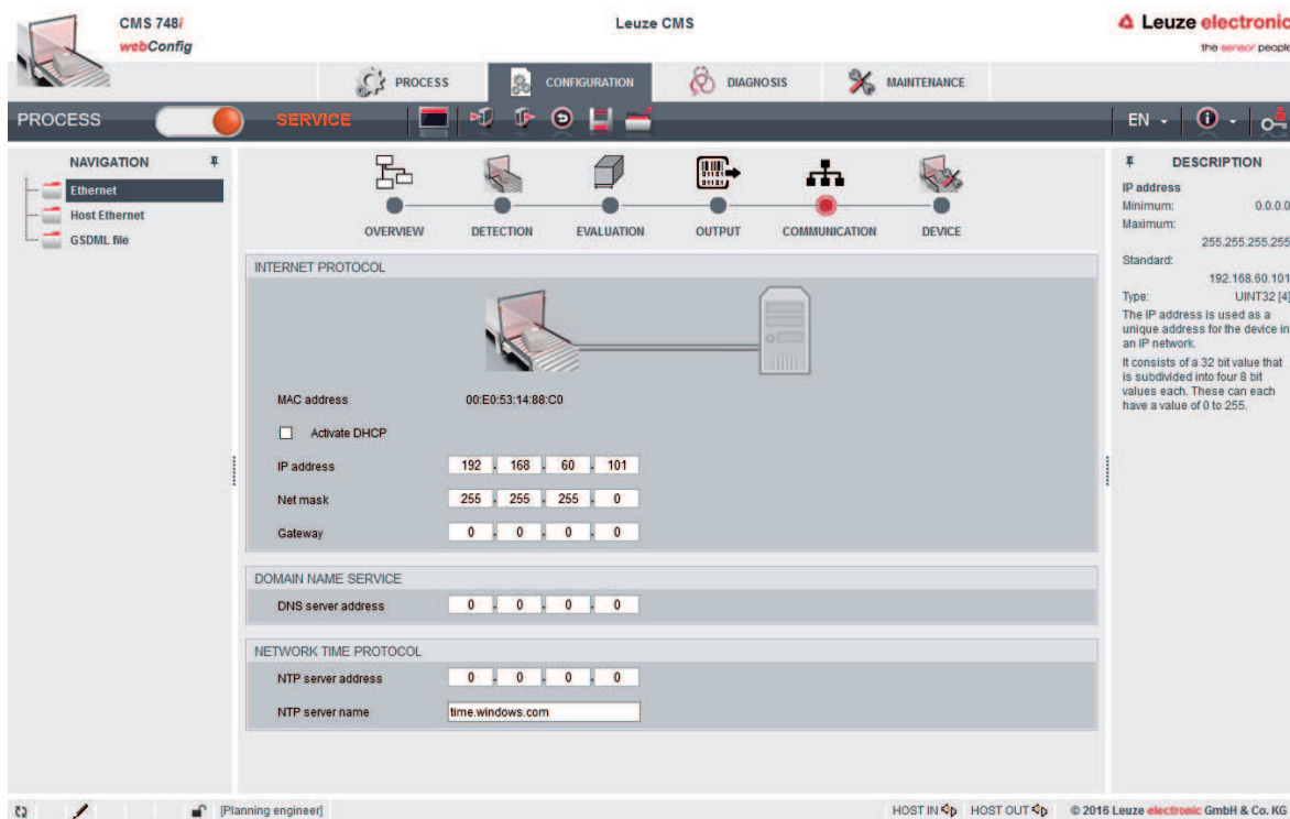
Fig. 8.10: Configuration of the Ethernet interface
