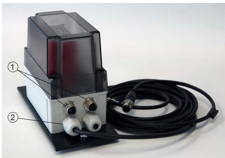
Figure 7.2: 426243 AC-ABF 70.A.1; acknowledgment unit with illuminated start button, on mounting plate, 5 m connection cable (MLDSET-M33 only)
