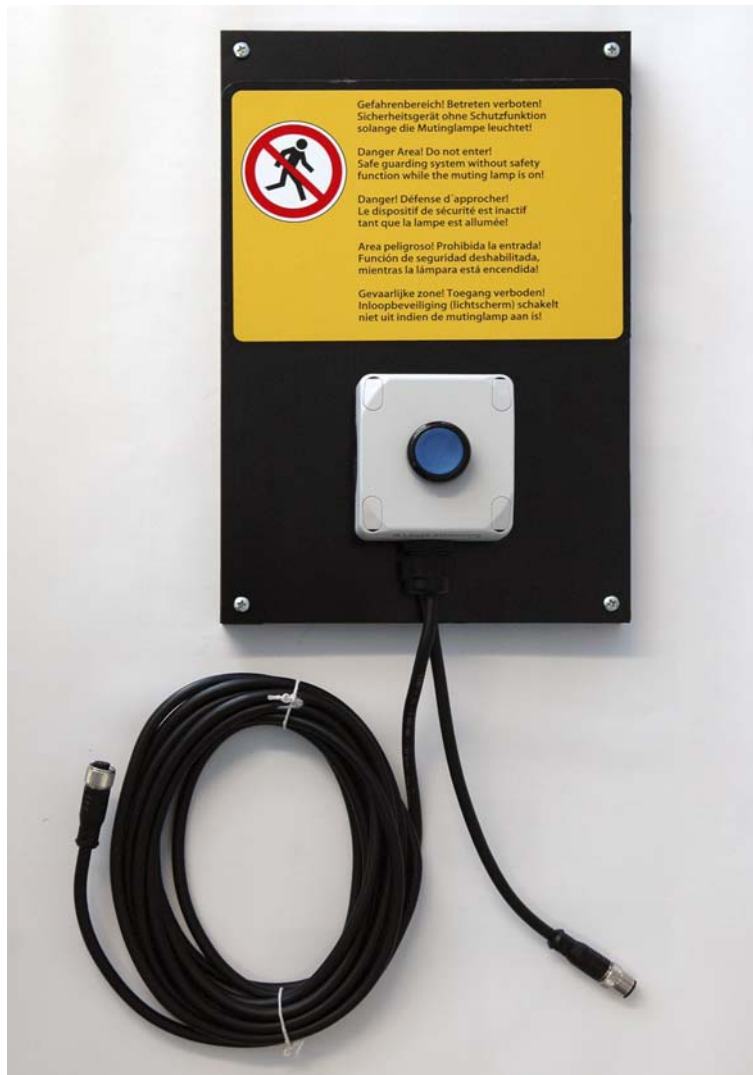
Figure 7.1: 426240 AC-ABF 70.BB; acknowledgment unit with illuminated start button, on mounting plate with notice sign in 5 languages, 5 m connection cable
