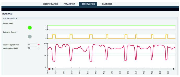
Simple visualization of the process data in the Leuze Sensor Studio PC configuration software enables a fast assessment of the process stability.
