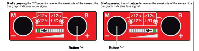
For an optimum setting, the displayed maximum and minimum signal must be symmetric about the switching point (middle of the bar graph).
