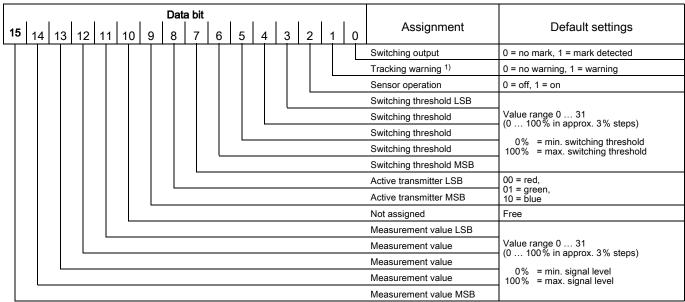
1) Only in combination with tracking function. For sensor versions without tracking function, this bit is not used.
