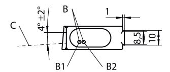
A Turning connector, turnable by 90°
