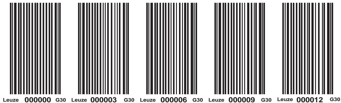
Fig. 16.5: contínua, grade de 30 mm
