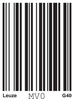
Figura 16.3: Etiqueta individual MV0, raster de 40 mm
