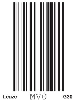
Figura 16.7: Etiqueta individual MV0, raster de 30 mm
