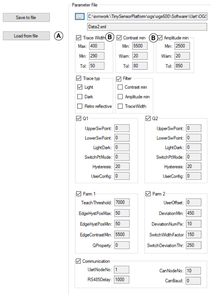
**A** Load parameters in sensor from file
