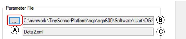
If a file is loaded, a comparison is made of all parameters on the sensor and in the file and the differences displayed in color.
