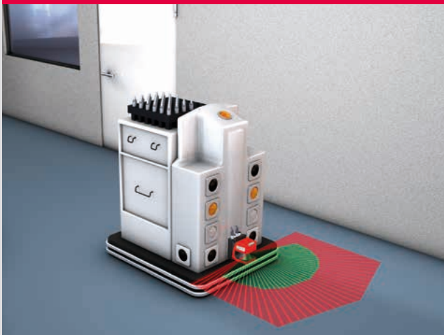
Collision protection of driverless transportation systems
