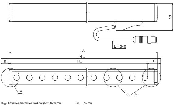
H<sub>PFN</sub> Nominal protective field height = 1500 mm
