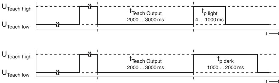
After the delay before start-up ( $\leq 300\text{ms}$ ) has elapsed, the teach button on the device can be operated.
