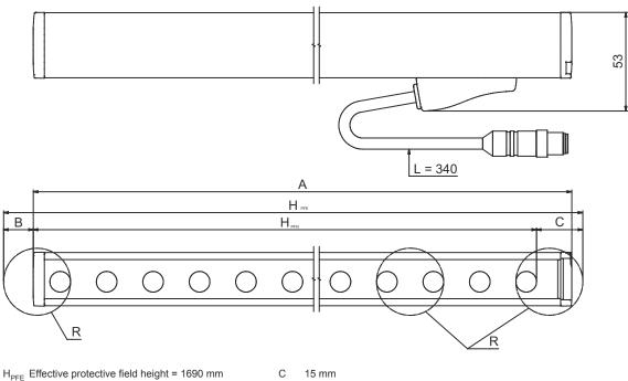
H<sub>PFN</sub> Nominal protective field height = 1650 mm
